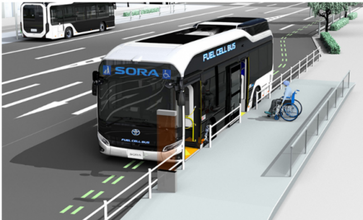
Image of automatic arrival control system
