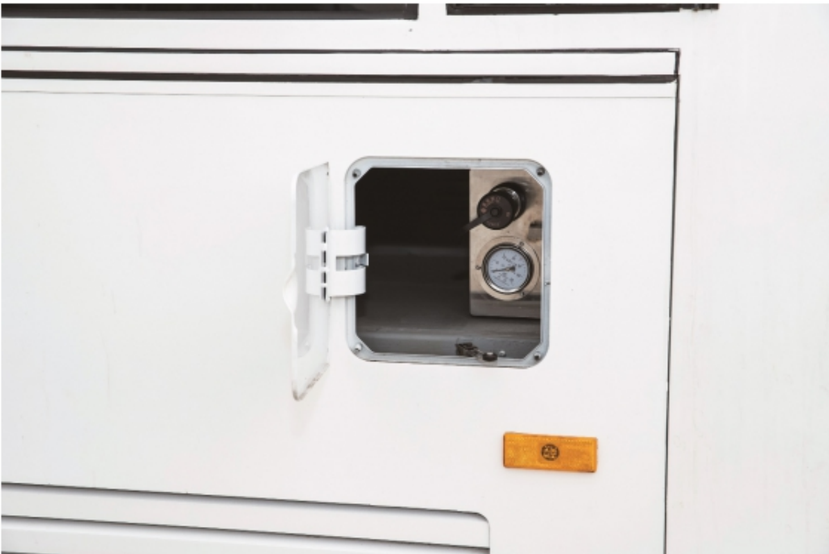
Hydrogen refueling panel provided with antistatic device - safe hydrogen refueling
