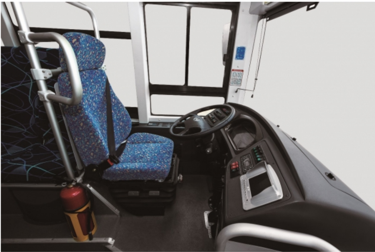
Adjustable damped driver seat - alleviating driver fatigue
