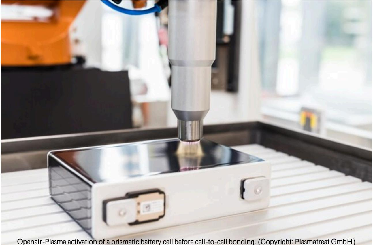
Openair-Plasma activation of a prismatic battery cell before cell-to-cell bonding. (Copyright: Plasmatreat GmbH)
