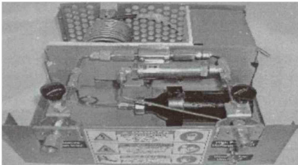
Fig. 7 The schematic diagram of metal hydride thermal compressor
