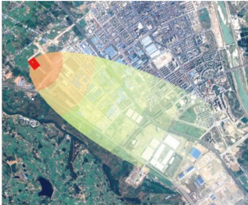
图 2 项目烟气排放效果示意图(主导风西北风) Fig.2 Drawings of Flue Gas Emissions ( Northwest Wind )
