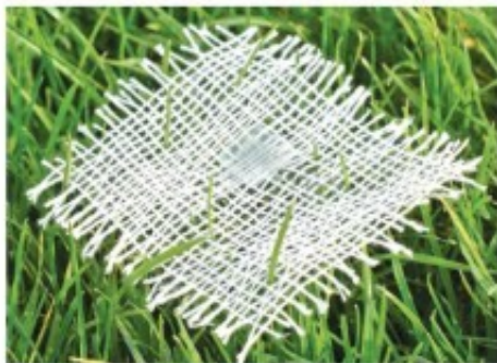
A solar cell textile integrated in a fabric.
